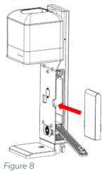
Press the ON/OFF switch to turn on the machine.
