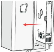
Open the battery compartment with the key and insert the battery in the slot.
